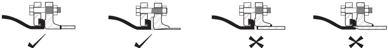
Flange bolts must not be overtightened, bolts should be tightened gradually and evenly and in a crosswise manner. Bolts should be positioned so that the bolt head is nearest the bellows to prevent the bolt damaging the bellows in service. Tightness of bolts should be checked approximately seven days after installation.
