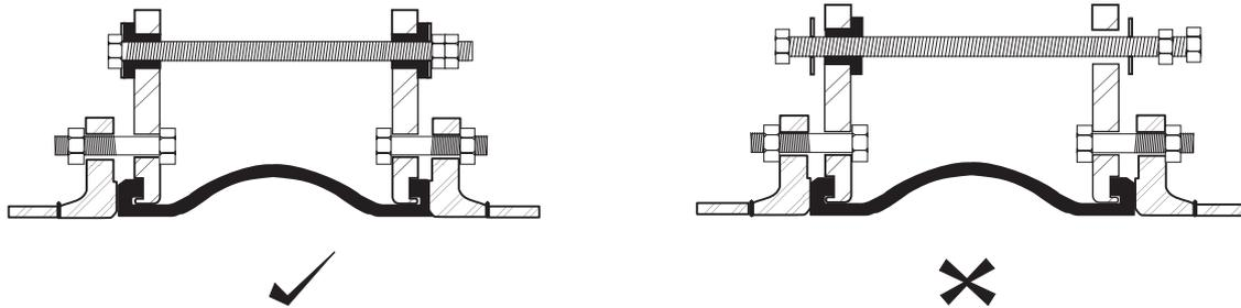
**Pressure Test.** If a hydraulic pressure test is to be carried out on a system containing rubber bellows ensure that the anchors are correctly fitted before the test is carried out. Also ensure that the test pressure (usually 1.5 x working) does not exceed the test pressure of the rubber bellows.
