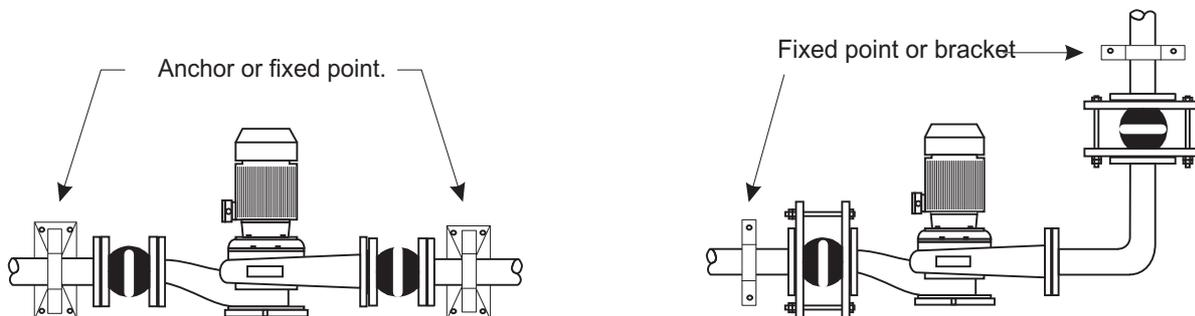
Rubber bellows will exert a pressure thrust in service and must be anchored to protect adjacent pipework and equipment. Rubber bellows will extend under pressure and must be anchored to prevent this happening.
